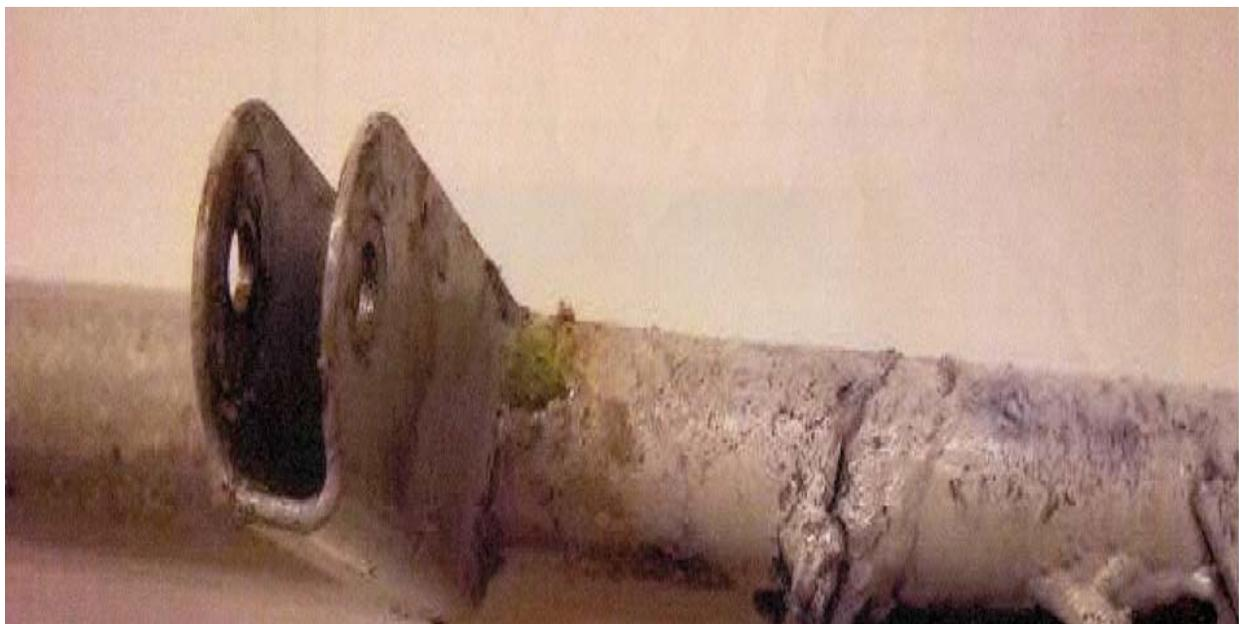
**Cessna: 550; Cracked Seat Belt Assembly**
