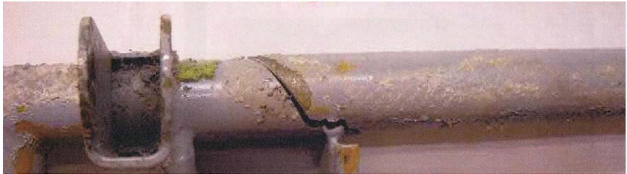
**Cessna: 550; Cracked Seat Belt Assembly**
